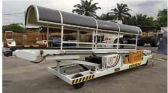
The unit has been design with walk behind motorised by hydraulic motor at the speed of 5km/h and built with anti collision system.
